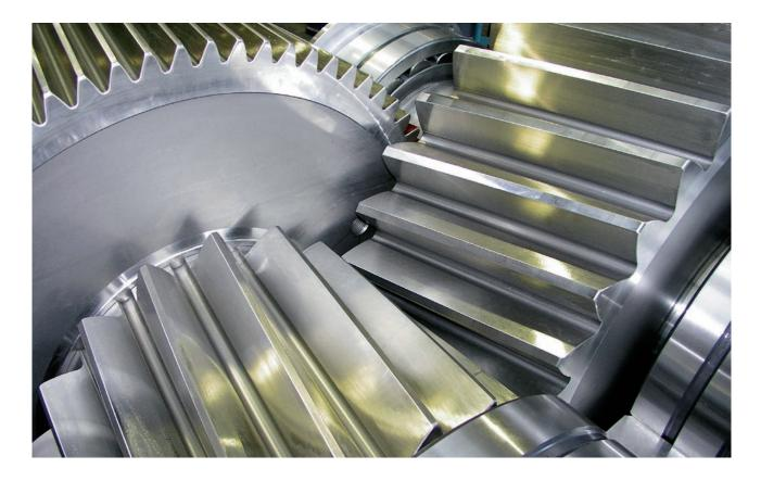
one-stage planetary gearbox. Eickhoff manufactures chain conveyor gearboxes up to size 65 for a maximum output torque of 650 kNm. Self-aligning sun gears ensure a uniform load distribution on the three planet wheels. A total of five different reduction ratios can be achieved by exchanging the first planet stage of the EP series or a spur stage of the EKP series.
