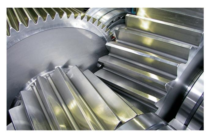
Eickhoff manufactures chain conveyor gearboxes up to size 65 for a maximum output torque of 650 kNm. Self-aligning sun gears ensure a uniform load distribution on the three planet wheels. A total of five different reduction ratios can be achieved by exchanging the first planet stage of the EP series or a spur stage of the EKP series.
